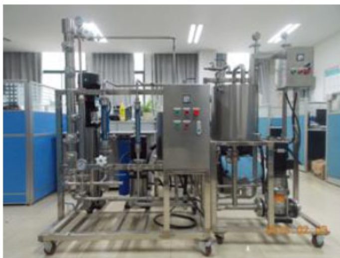
Fig. (3.2). The equipment of membrane separation with ultrasonic.
