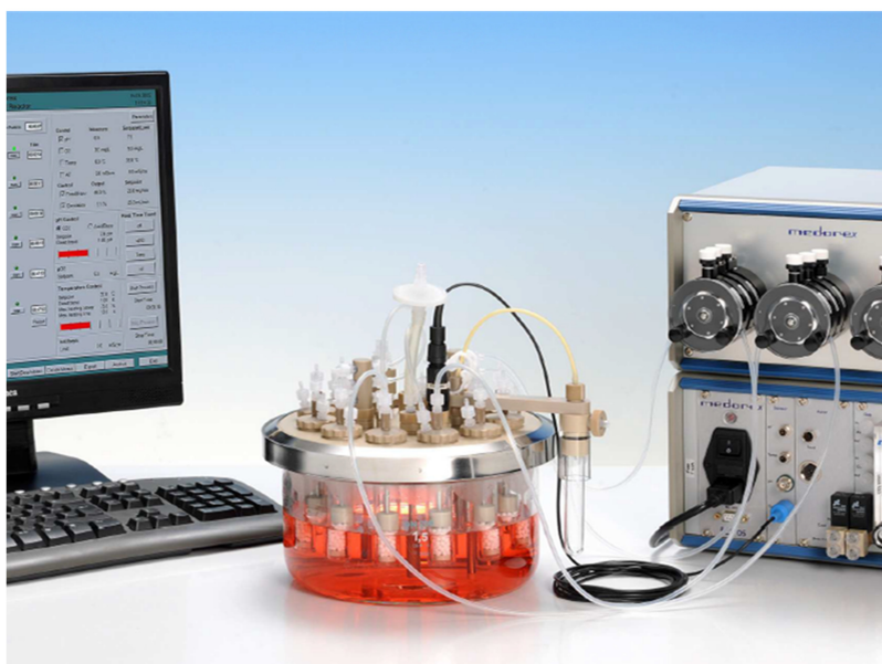
Fig. (1). The Multiferm multi-fixed-bed fermenter system. Middle: Conditioning vessel with the 12 single fixed-bed units. Left: Process control system WinErs. Right: Control unit for feed, harvest, pH, aeration and temperature (medorex e.k., with kind permission).
