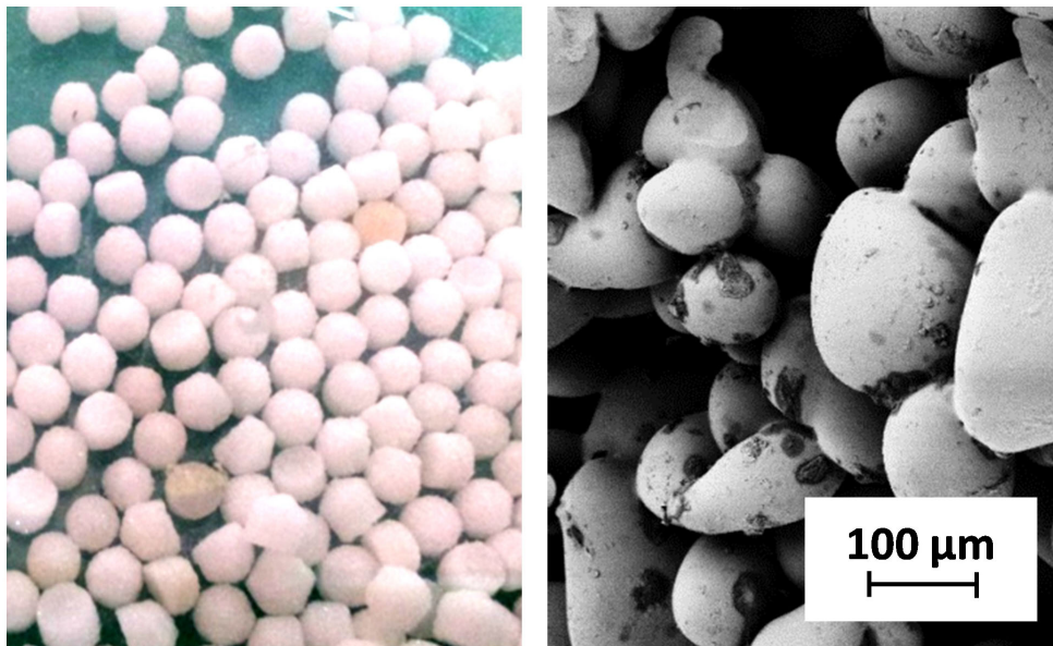
Fig. (3). Top: VitraPOR® carrier with a diameter of 4 mm. Bottom: SEM image with 250-fold magnification (scale is 100 μm).
