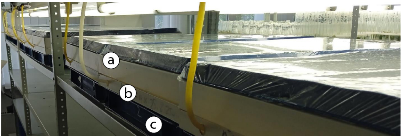
Fig. (1). Construction of a flow-through hydroponic system: a - hydroponic tray, b - frame with non-woven fabric, c - translucent cover.
