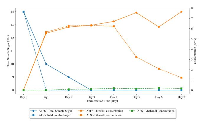
Fig. (6). Changes in sugar, ethanol, and methanol concentration of nipa sap during closed and open vessel fermentation over time.
