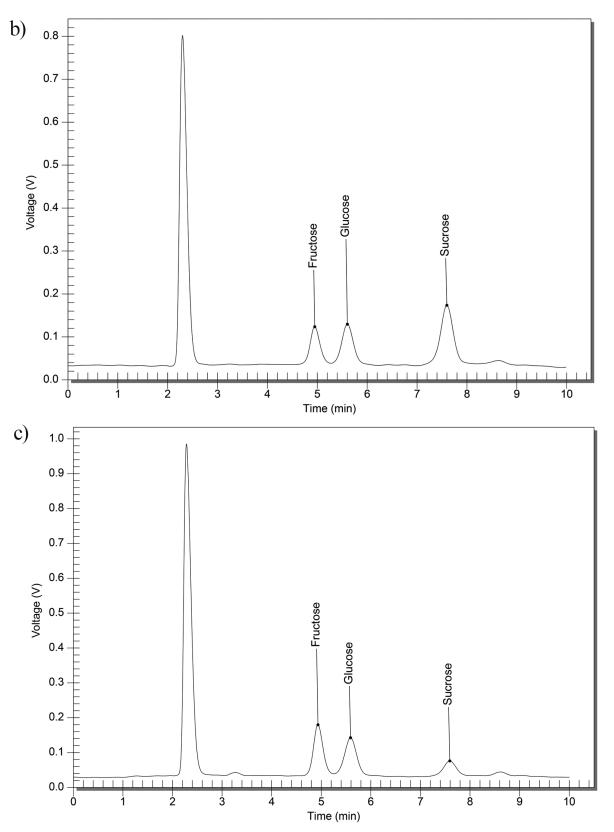
Fig. (3). Chromatograph of specific sugar content of (a) FNS1 (b) FNS2 and (c) FNS3.
