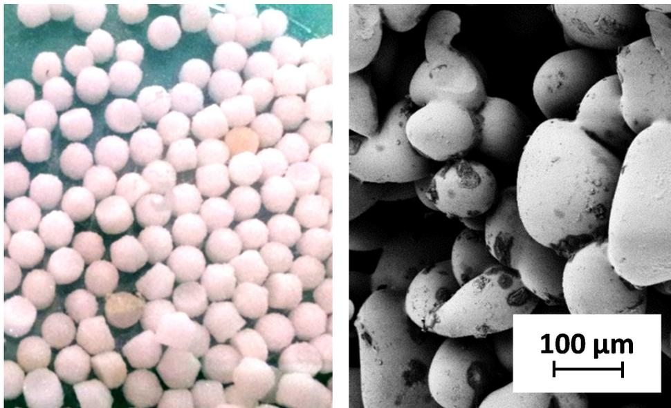
Fig. (3). Top: VitraPOR<sup>®</sup> carrier with a diameter of 4 mm. Bottom: SEM image with 250-fold magnitude (scale is 100 μm).
